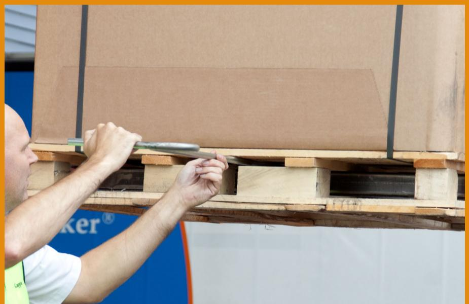
**6.** With the first shipment of the Conicube, you will receive a long key, which operates the valve. This special key has four equal, special shaped sides. Align this key with the inside profile of the spindle of the valve. Insert the key in the spindle until it reaches the end of the hole.
