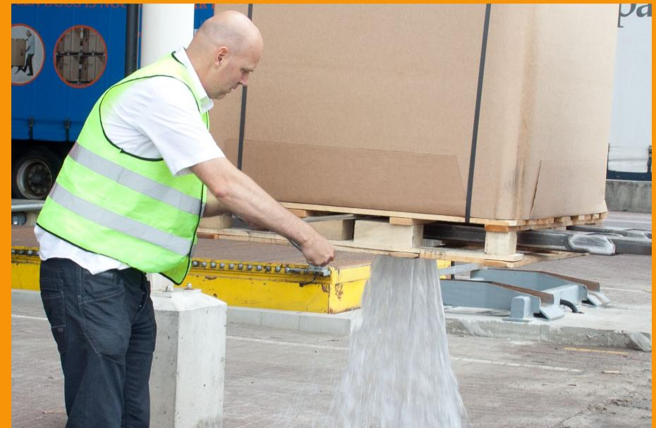
**8.** The speed of the discharge depends on the viscosity of the product. The unit will empty completely and very little product is left in the unit. If desired the last bit can always be squeezed out later, when the bag has been removed from the unit.
