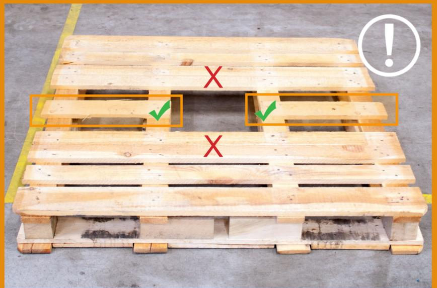
**7.** Place the unit with cassette on the pallet and make sure the open spaces in the positioning plate fall directly in the top shelves in the center of the pallet. The unit will then always be positioned correctly on the pallet.
