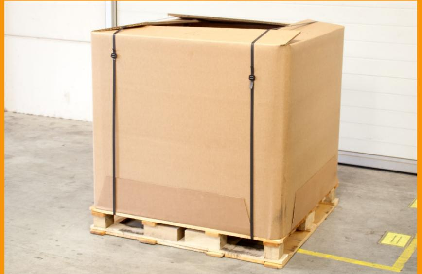
**11.** Tie the small white corner ropes located at the corners of the bag (pulled out in step 9) to the two straps that have just been placed on the unit. This holds the bag up so it is easier to fill, and later the receiver will be ensured this way that the bag cannot fall down on the valve during discharge and block the discharge opening.
