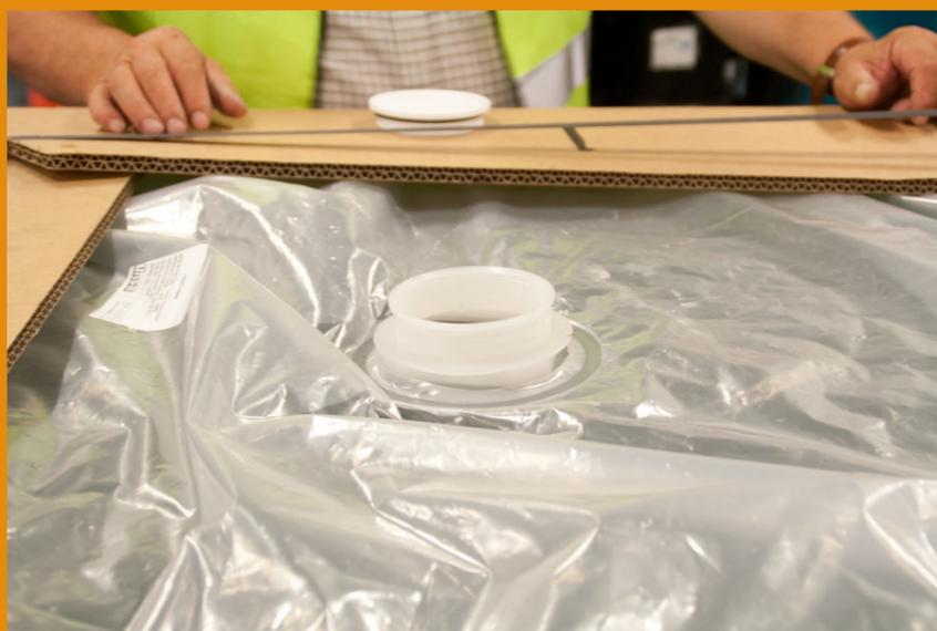
**3.** When full, place the cap back on the filling opening. Remove the filling bridge, if that has been used.
